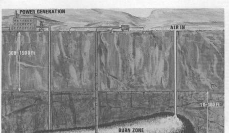
TYPICAL *IN SITU* COAL GASIFICA-TION SITE — On the surface, product gas can be burned to generate electricity on-site, used as a chemical feedstock, or upgraded to synthetic natural gas.
